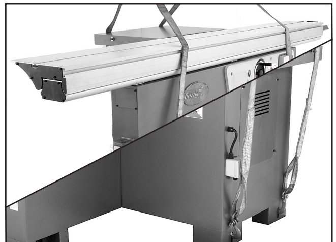
Figure 17. Lifting the saw base unit.
